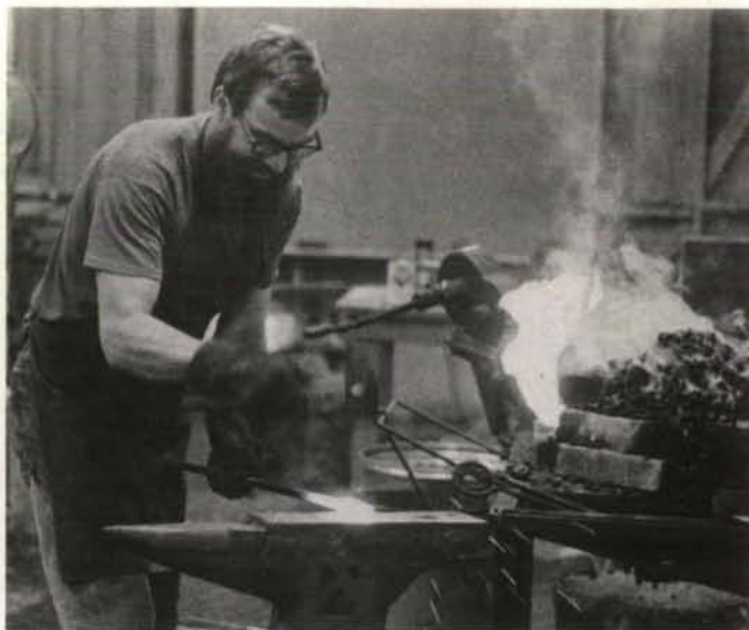
Blacksmithing student Ronald Baker flattens a piece of hot metal while learning the process for making Damascus Steel.
