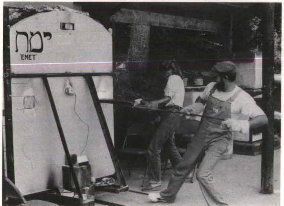
Roxie Thomas pulls out a scorching peep brick as Wayne Horton deposits rock salt in the kiln during a salt-firing.
