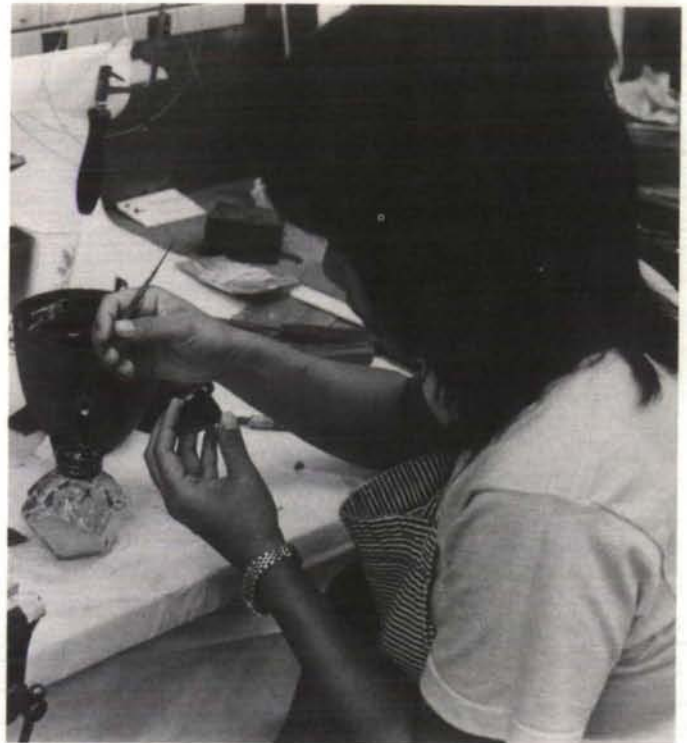
Metal student Mei-Kwang Lu prepares a wax model for the lost wax casting class.
