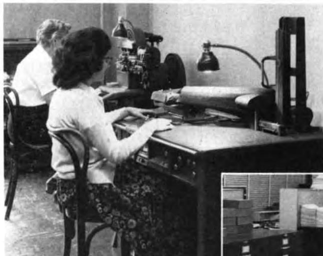
The Graphotype (far side) and Addressograph machines. The former makes the addressograph plates. The ARROW run is done on the Addressograph (takes 2 1/2 days) and we use it for addressing mailing labels and envelopes.
